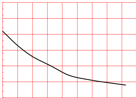
FIG.7: Relative variations of gate trigger current, holding current and latching current versus junction temperature
