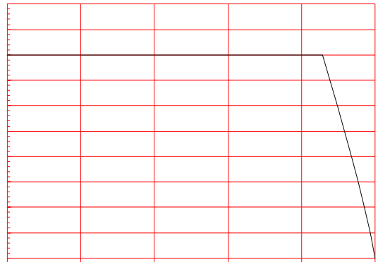
FIG.2: RMS on-state current versus case temperature
